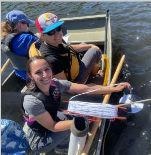
Taking water depth and water visibility reading with the Secchi Disk.
