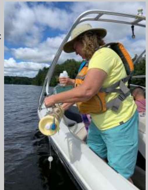
Taking a water sample from deep in Rainbow Reservoir using a Van Dorn water sampler.
